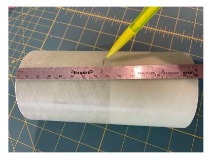
4) MEASURE AND MARK THE HALFWAY POINT ON THE OUTSIDE OF THE COUPLER.
