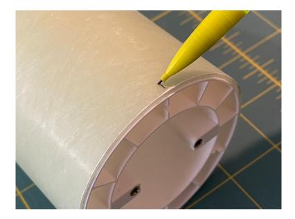
2) IF INSTALLING (3) GROMMETS, UTILIZE THE NOTCHED RIBS ON THE INSIDE OF THE SLEEVE FOR EVEN SPACING. IF INSTALLING (2) GROMMETS, UTILIZE THE RIBS LOCATED IN LINE WITH THE SLED MOUNTING ARMS. MARK THESE LOCATIONS ON THE COUPLER.
