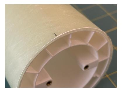
3) APPLY A LIGHT COAT OF EPOXY TO THE INSIDE OF THE COUPLER - APPROXIMATELY AN INCH WIDE BAND WORTH (CAREFUL - A LITTLE GOES A LONG WAY!) AND INSTALL THE SLEEVE INTO THE COUPLER, AGAIN FLUSH WITH THE END. A CLEAR THIN 30-MIN EPOXY WORKS GREAT.
