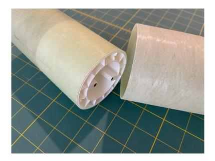
1) INSERT THE SLEEVE INTO THE NOSE CONE COUPLER - FLUSH WITH THE END THAT WILL BE INSERTED INTO THE NOSECONE. DO NOT EPOXY THE SLEEVE IN PLACE YET!
